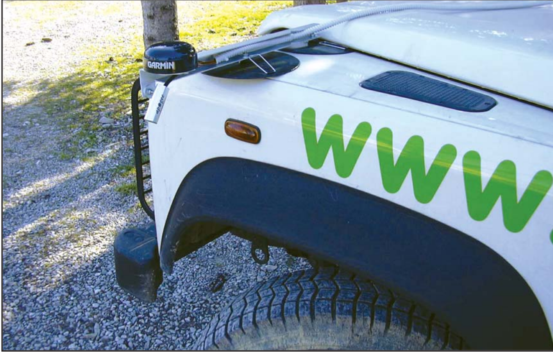
The sensors mounted on the front of the roadmap vehicles are a Garmin® geographic position sensor and an IRTS precision infrared thermometer (silver cylinder pointed downward at an angle).
