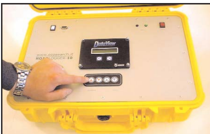
A CR10X is embedded in a protective travel case; data are accessed via a DataView display
