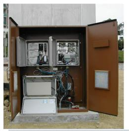
SDMX50 TDR multiplexer, and TDR100 reflectometer. The datalogger polled two horizontal TDR cables every four minutes and compared the reflected waveform to a baseline signature. If the reflected
