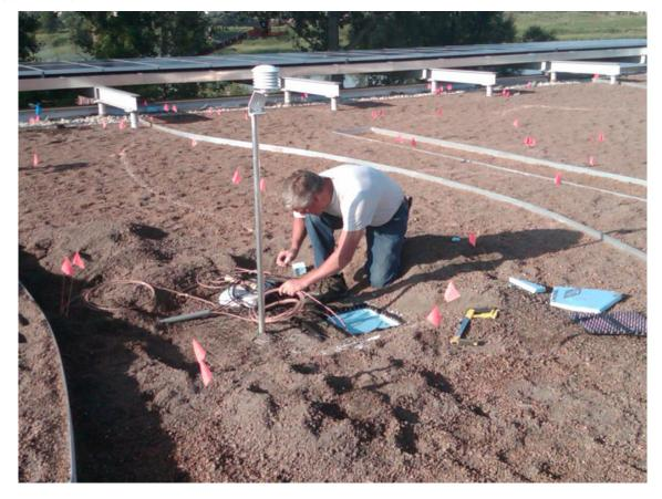
Campbell dataloggers control weather and soil condition monitoring for roof-garden research
