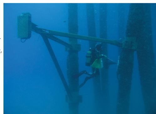
Sensors mounted 5m below the surface measure the oceanographic parameters.
