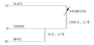
FIGURE 7-1. 107 Thermistor Probe Schematic
