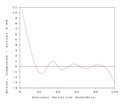
FIGURE 2. Relative Humidity Sensor Polynomial Error Curve
