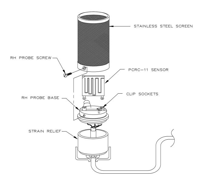
FIGURE 4. 207 Probe Assembly Drawing
