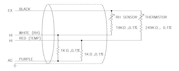
FIGURE 3. 207 Probe Schematic
