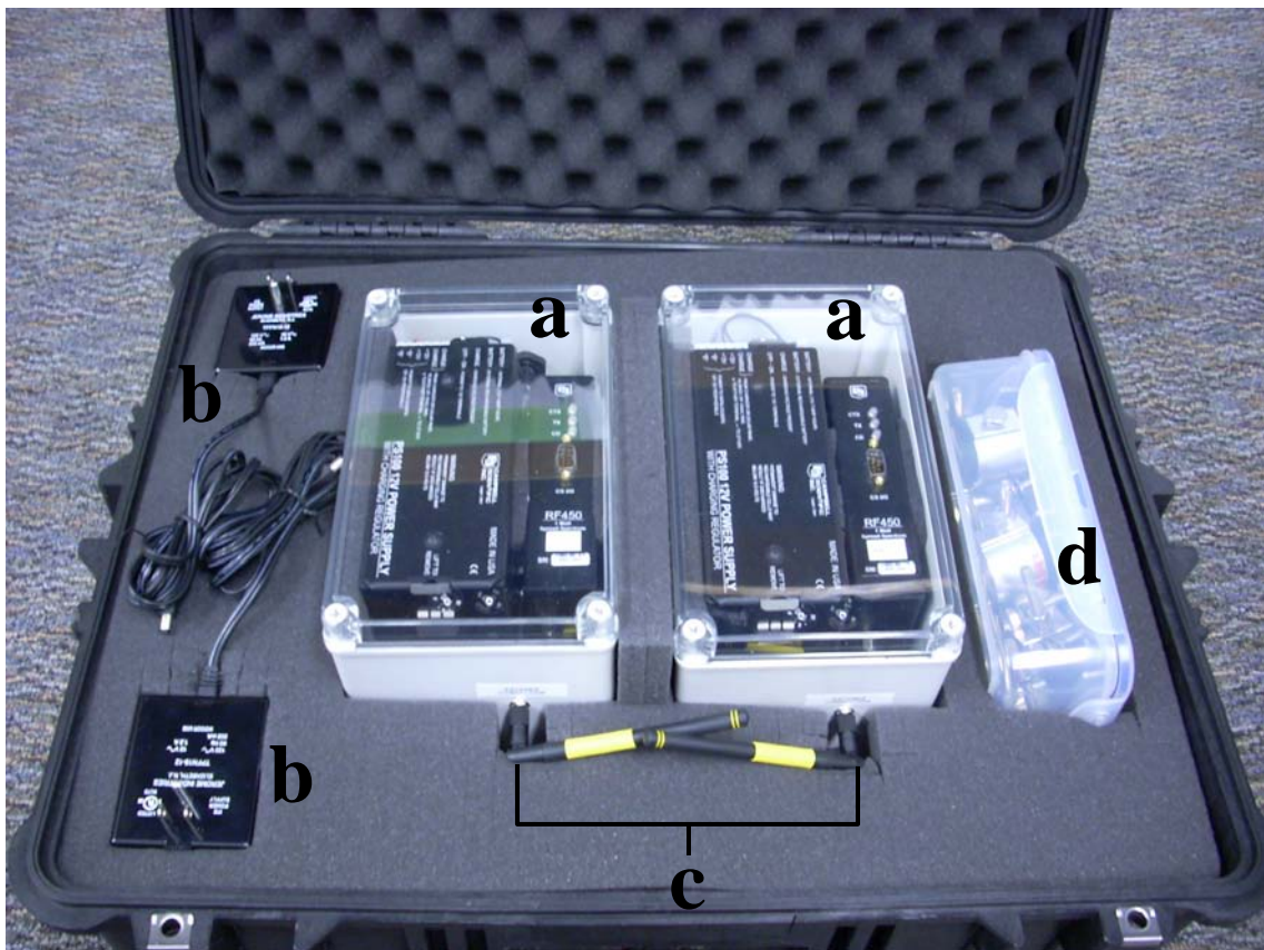
FIGURE 1-1. Top layer of the box contains two (a) plastic enclosures housing the RF450 radio and PS100 Power Supply; two (b) 15966 wall chargers; two (c) 19512 whip antennas; (d) box holding antenna mounting brackets; and diagnostic CD (sits next to (d)).
