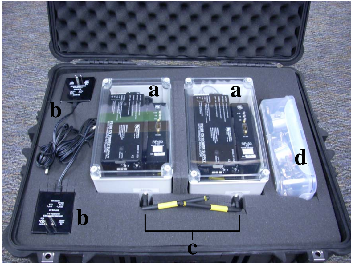
FIGURE 5-3. The top layer contains two (a) plastic enclosures housing the RF450 radio and PS100 Power Supply; two (b) 15966 wall chargers; two (c) 19512 whip antennas; (d) box holding antenna mounting brackets; and diagnostic CD (sits next to (d)).
