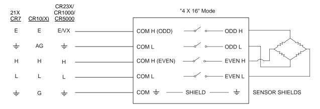
FIGURE 15. Full Bridge Measurement
