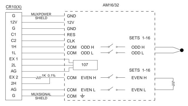
FIGURE 20. Thermocouple and Soil Block Measurement
