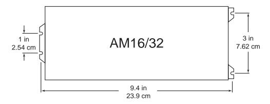
FIGURE 21. Mounting Tab Hole Pattern
