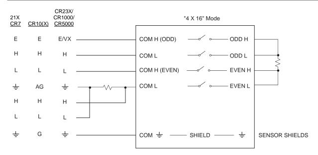
FIGURE 14. Four Wire Half Bridge Hook-up and Measurement
