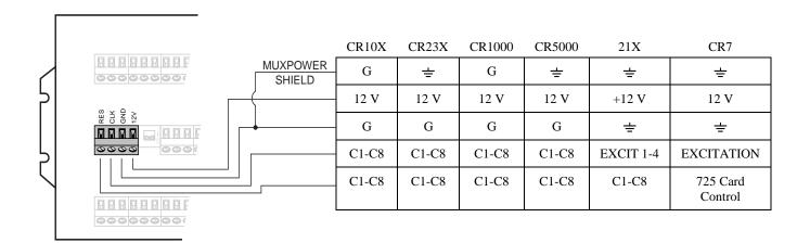
FIGURE 3. AM16/32 to Datalogger Power/Control Hookup
