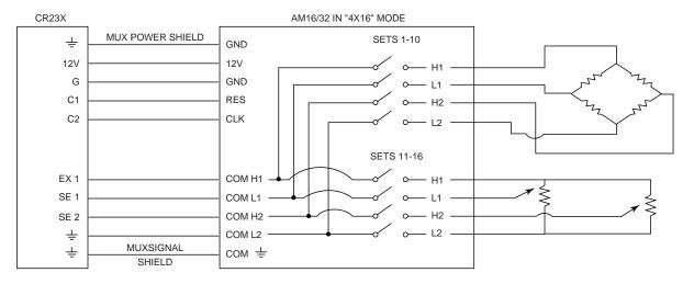
FIGURE 9. Wiring Diagram for Strain Gages and Potentiometers
