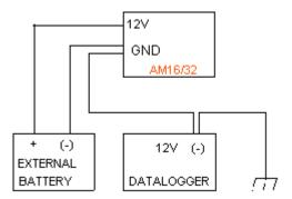
FIGURE 4. Power and Ground Connections for External Power Supply.
