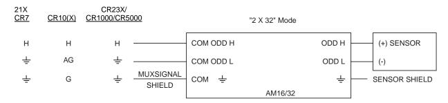
FIGURE 10. Single-ended Measurement without Excitation
