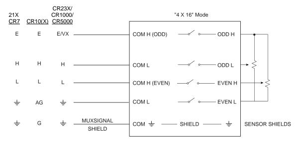
FIGURE 13. Potentiometer Hook-up and Measurement
