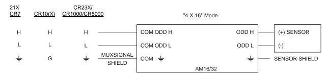
FIGURE 11. Differential Measurement without Excitation
