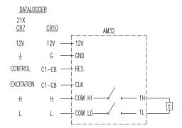
FIGURE 5-2. Differential measurement.
