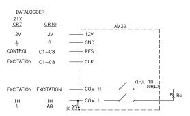
FIGURE 5-3. Half Bridge measurement with resistor at the datalogger.
