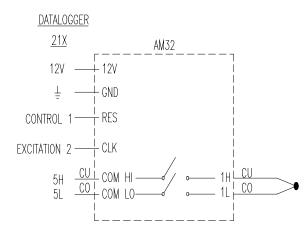
FIGURE 7-2. Wiring Diagram for 21X and Thermocouples with reference at the datalogger.
