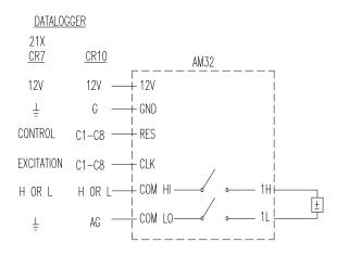
FIGURE 5-1. Single-Ended Measurement
