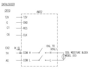
FIGURE 7-1. Wiring Diagram for CR10(X), AM32 and 223 Soil Moisture Block example.
