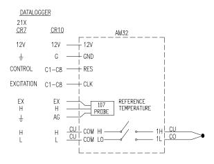
FIGURE 6-2. Differential thermocouple measurement with reference junction at the AM32.
