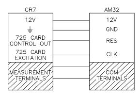
FIGURE 3-1. Hook-up diagrams for datalogger to AM32 connections.
