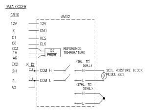
FIGURE 7-3. Wiring Diagram for example of CR10(X) measuring soil moisture blocks and thermocouples with reference temperature at the AM32.
