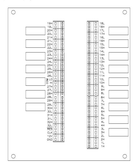
FIGURE 1-1. Plan view of the AM32 Relay Multiplexer with cover plate removed.
