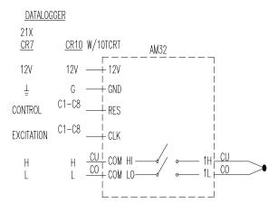
FIGURE 6-1. Differential thermocouple measurement with reference junction at the datalogger.
