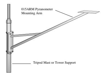
FIGURE 3-2. 015 Pyranometer Mounting Arm
