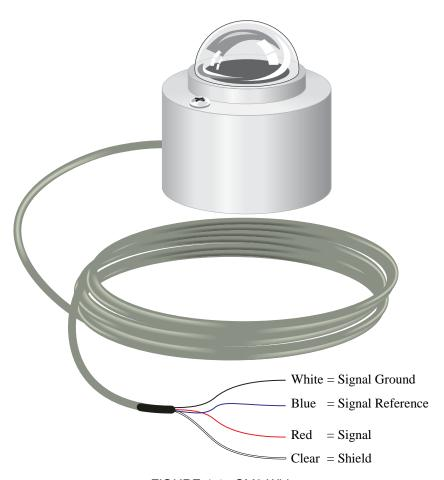
FIGURE 4-1. CM3 Wiring
