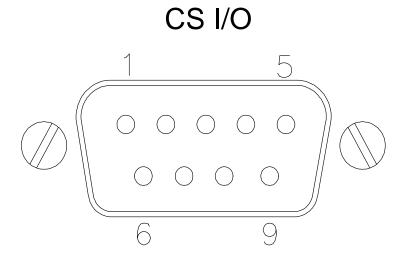
FIGURE E-1. COM310's Male 9 Pin Connector
