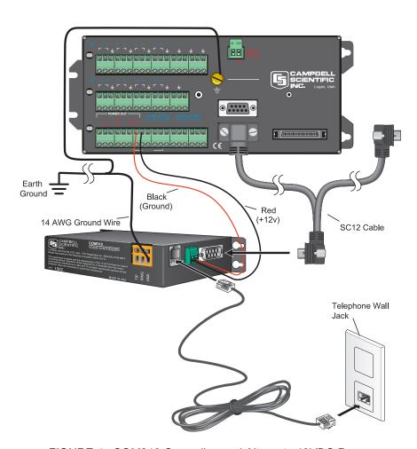
FIGURE 4. COM310 Grounding and Alternate 12VDC Power
