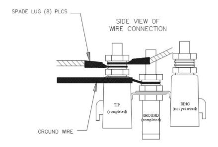
FIGURE 6. Side View of Surge Suppressor Wiring
