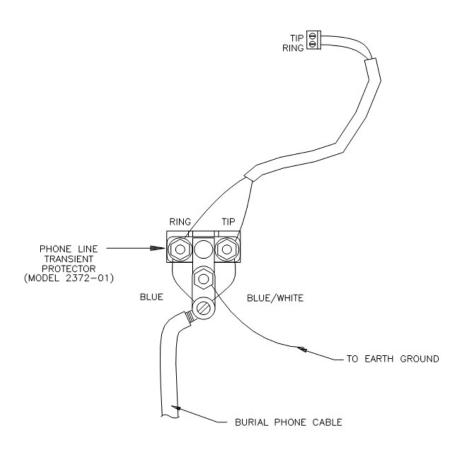
FIGURE 5. Top View of Surge Suppressor Wiring
