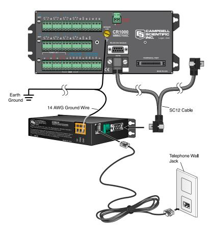
FIGURE 2. COM310 Hardware Connection Using Standard RJ11
