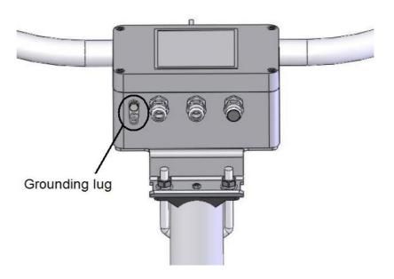
The CS120 must be properly grounded by taking a ground wire with a minimum cross sectional area of 6 mm<sup>2</sup> and maximum length of 5 m from the brass grounding lug in the lower face of the electronics enclosure to an adequate grounding point. The pole and foundations of a pole mounted installation will provide some basic lightning protection and protection against radio frequency interference and should also be correctly grounded.
