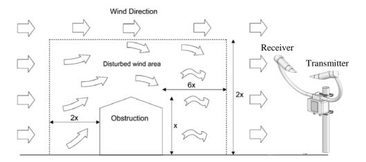
In order to reduce the service frequency with the unit, the CS120 should be placed away from sources of contamination, in the case of roadside monitoring; larger mounting poles can be used. More regular maintenance will be required when the instrument is placed in areas where contamination is unavoidable or where measurements may be safety critical.
