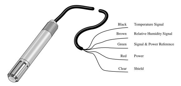
FIGURE 5. CS500 Wiring
