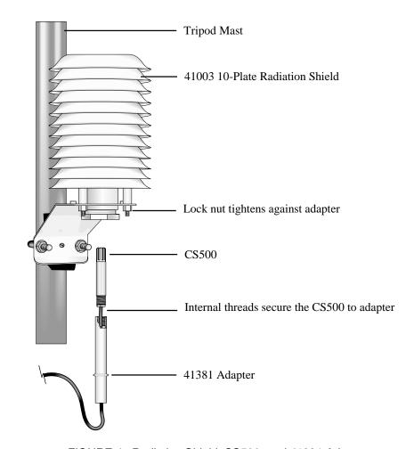
FIGURE 4. Radiation Shield, CS500, and 41381 Adapter
