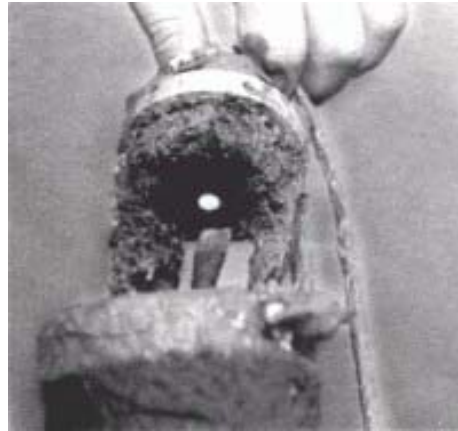
FIGURE 5-1. Preventing Bio-fouling of the CS510-L
