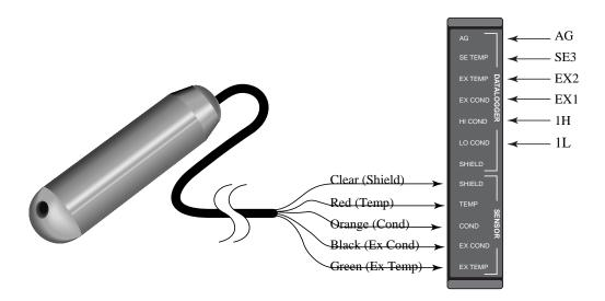
FIGURE 4-1. CS547 Wiring Diagram for Example Below
