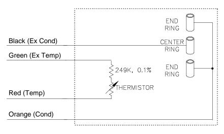
FIGURE 13-1. CS547 Conductivity and Temperature Circuit Diagram
