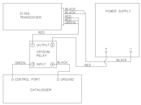
FIGURE 5-1. DC1765 Wiring
