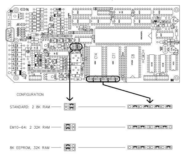
FIGURE H-2. Jumper Settings for Different RAM Configurations
