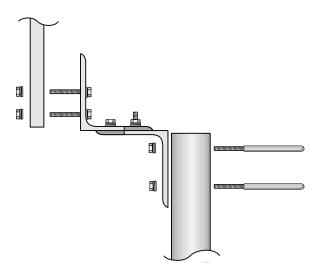
FIGURE 6.3-1. Antenna Mounting Hardware, Exploded View
