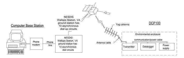
FIGURE 2-1. Data Retrieval Diagram
