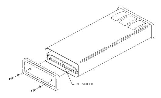
FIGURE H-1. Disassembling CR10
