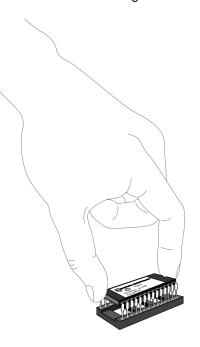
FIGURE I-6. Inserting the New PROM
