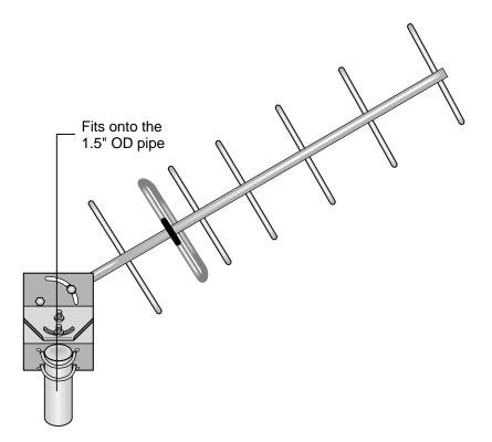
FIGURE 6.3-2. Antenna Mounting Hardware, Assembled View 1
