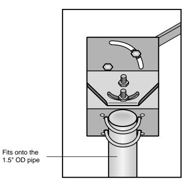
FIGURE 6.3-3. Antenna Mounting Hardware, Assembled View 2
