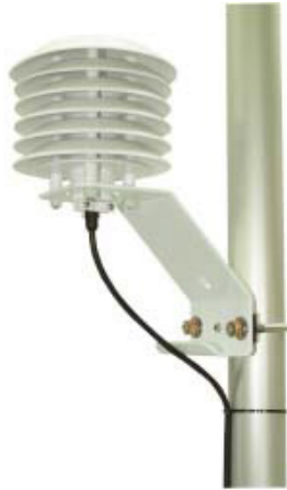
FIGURE 6-11. Solar radiation shield with EC150 temperature probe
