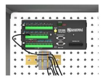
Figure A-6. An installed and wired 006706-002 DIN-Rail Terminal Kit
