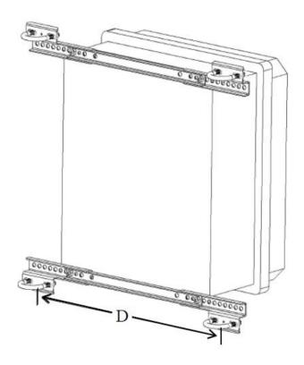
Figure 7-4. Enclosure brackets configured for a tower mount.
