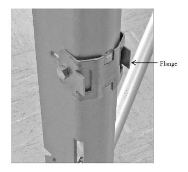
Figure 7-7. The #19124 bracket attached to a CM110 tripod.
