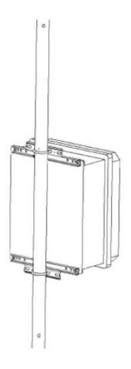
Figure 7-3. An enclosure attached to a tripod mast.
