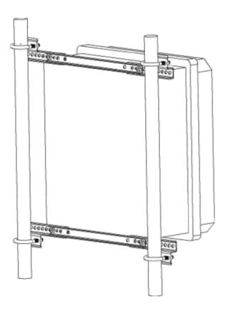
Figure 7-6. An enclosure attached to two tower legs.
