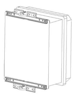
Figure 7-1. An enclosure with the mast mounting option attached to a tripod mast via u-bolts.
