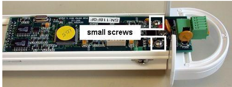
FIGURE A-4. Location of Small Main Board Screws
