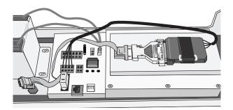
FIGURE 3.3-4. Short-Haul Modem Mounting and Connection
