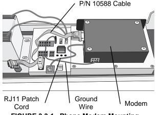
FIGURE 3.3-1. Phone Modem Mounting and Connections
