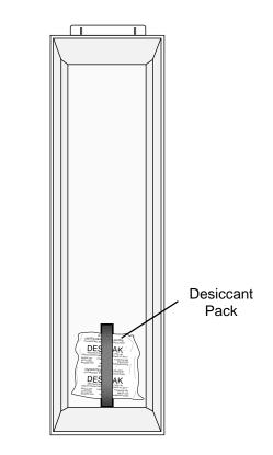
FIGURE 3.4-1. Desiccant Installation
