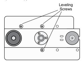
FIGURE 4.2-2. Leveling the Pyranometer
