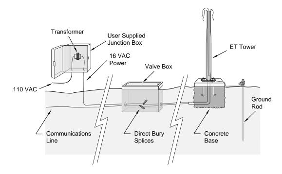
FIGURE 2.1-1. ET Tower Installation
