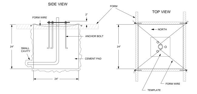
FIGURE 2.1-2. ET Tower Base Installation
