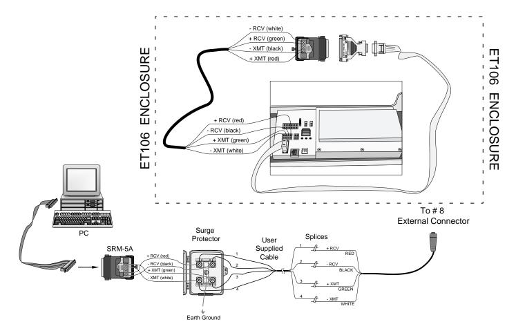
FIGURE 3.3-5. Short-Haul Modem Wiring Diagram
