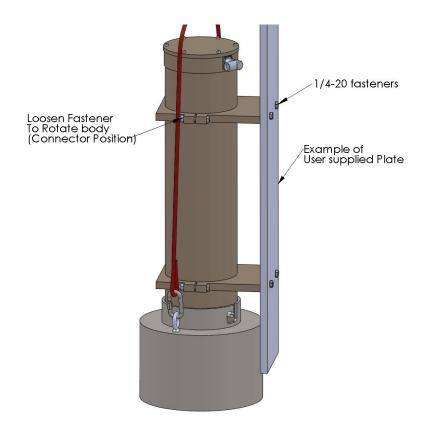
FIGURE 4. Example of Wall/Plate Mounting
