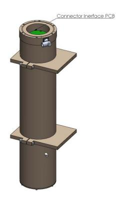
FIGURE 10. GMON3 with Top Cap Removed
