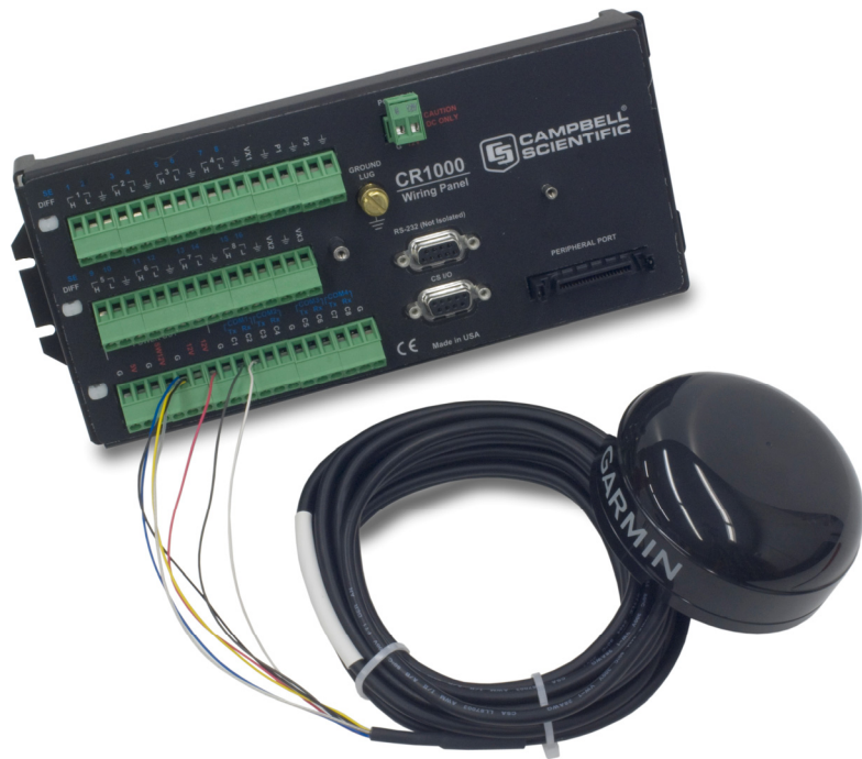
FIGURE 2. CR1000 to GPS16X-HVS connection
