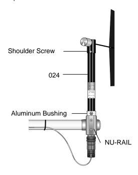
FIGURE 4.3-1. Met One 024A Wind Direction Sensor
