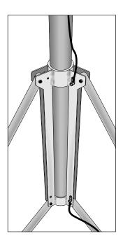
FIGURE 2-5. Tripod Ground Connections
