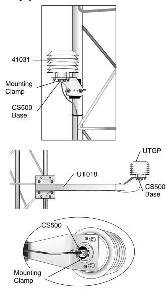
FIGURE 4.10-1. CS500 Temperature and RH Probe
