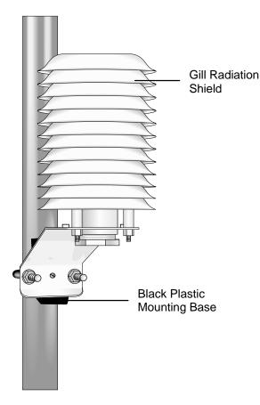
FIGURE 2-10. Gill Radiation Shield
