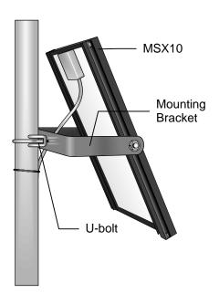
FIGURE 3.1-6. MSX10 Solar Panel on CM6 or CM10 Tripod
