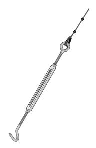
FIGURE 2-8. Turnbuckle Assembly
