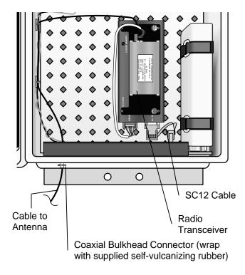
FIGURE 3.3-5. RF95 RF Modem and RF100/RF200 Transceiver
