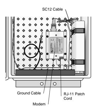
FIGURE 3.3-2. Telephone Modem Installation
