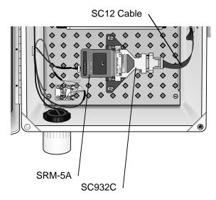
FIGURE 3.3-4. SRM-5A and SC932C in MetData1
