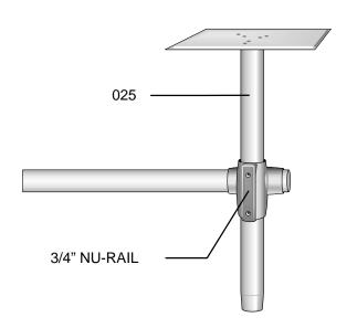
FIGURE 2-12. 025 Pyranometer Crossarm Stand
