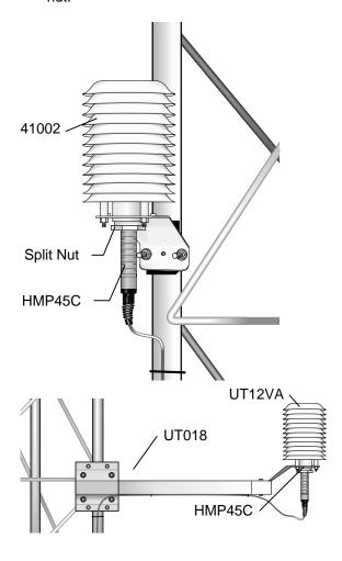
FIGURE 4.11-1. HMP35C Vaisala Temperature and RH Probe
