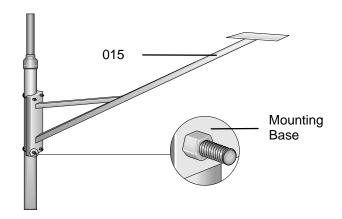
FIGURE 2-11. 015 Pyranometer Mounting Arm
