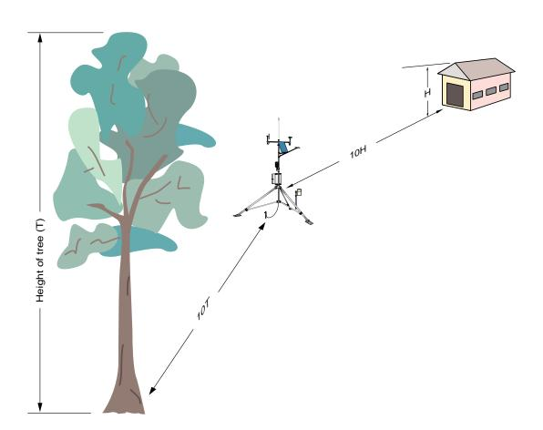
FIGURE 1.3-1. Effect of Structure on Wind Flow
