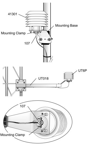
FIGURE 4.8-1. 107 Temperature Probe
