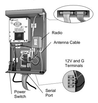
FIGURE 3.3-6. RF232 Base Station Installation
