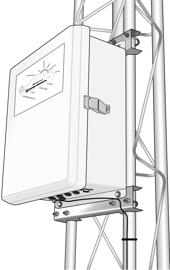
FIGURE 3.1-2. MetData1 Enclosure on UT10 or UT30 Tower
