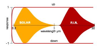
FIGURE 3. Approximate Spectral Sensitivity and Solar/F.I.R. Radiation
