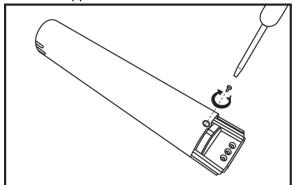
4. Install the 4-40 x ½ SS slot head screw supplied with the copper sleeve. Tighten the screw until snug. The hex screw is no longer needed.
