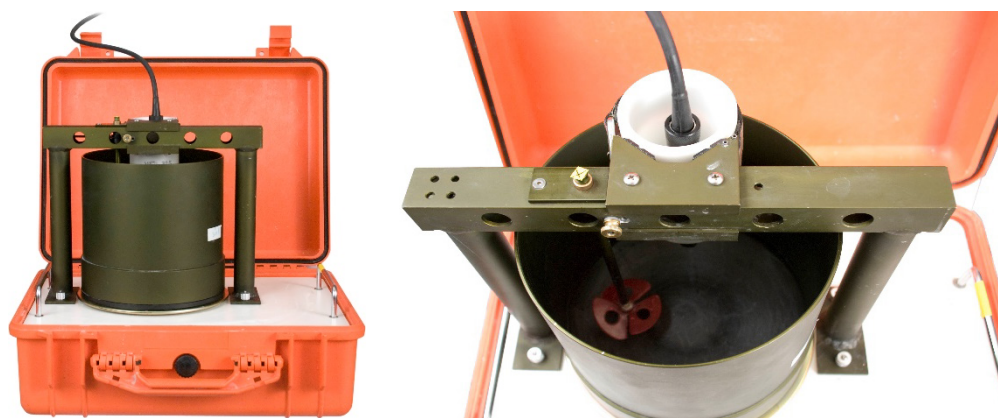
FIGURE 7-8. Portable Sediment Suspender (left) and OBS beam orientation in suspender tub (right)
