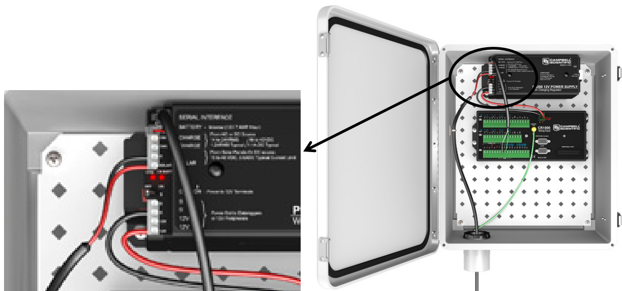
FIGURE 2-2. The PS200 connected to a CR1000 and solar panel
