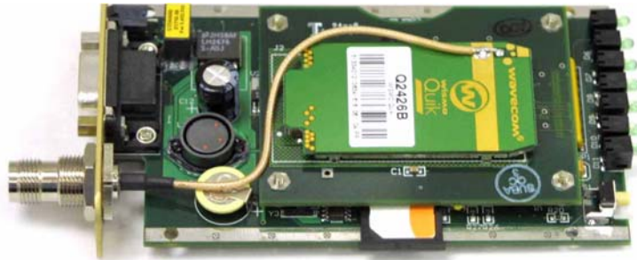
FIGURE B-6. Inserting the SIM
