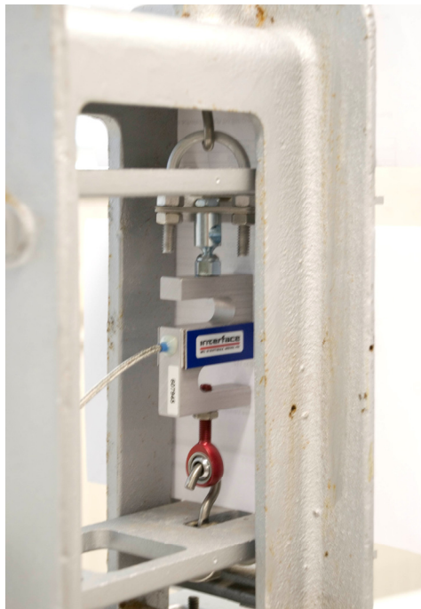
FIGURE 3.2-6. Side view showing cable and arms horizontal and overload protection screw.
