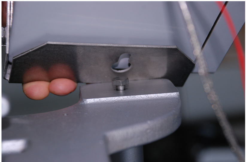
FIGURE 3.2-2. Keyholes aligned over bolts.
