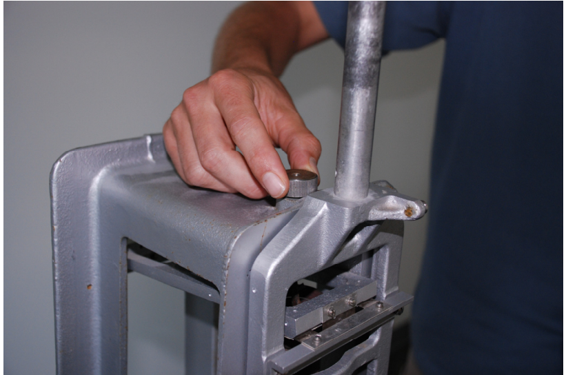
FIGURE 3.1-5. Unscrewing zero adjustment knob.
