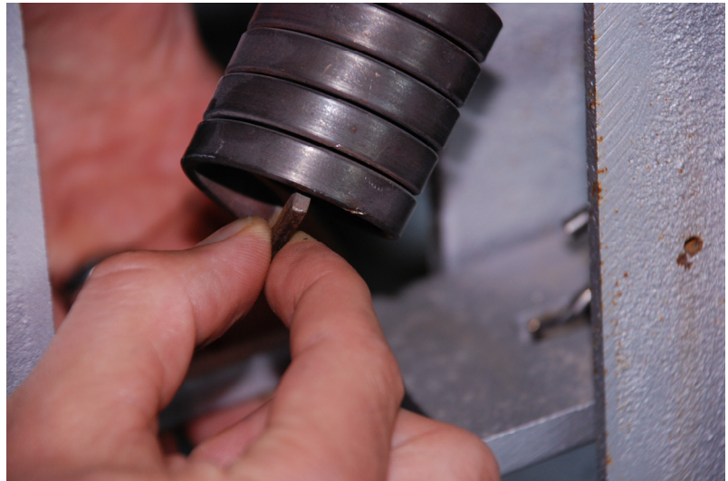
FIGURE 3.1-6. Removal of helical spring.
