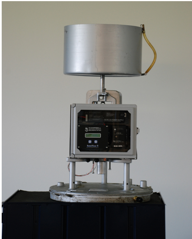
FIGURE 3.2-4. Properly installed internal enclosure. Notice it is slightly shifted to the right.
