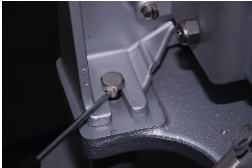
FIGURE 3.1-3. Bolts that will be loosened to remove punch assembly and tape reel assembly.
