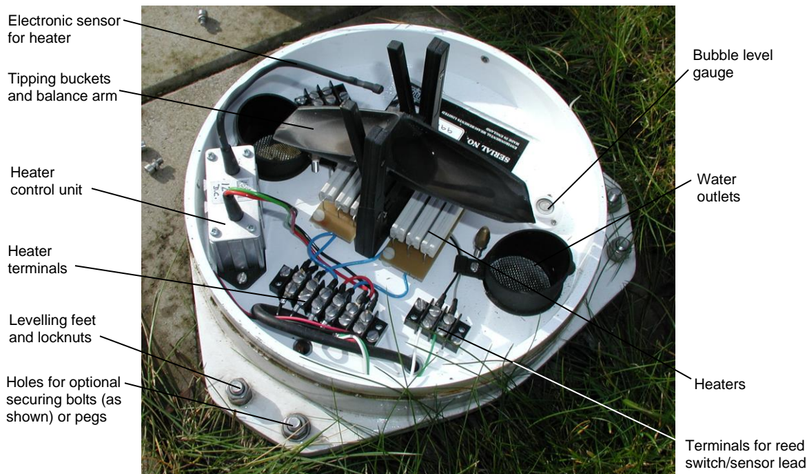
Figure 4. Internal View of SBS500H (Heated Version)
