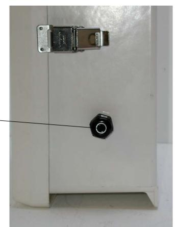
IRDA Sensor fitted to enclosure using a high-quality cable gland
