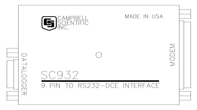
FIGURE 1. SC932 9-Pin to RS-232-DCE Interface
