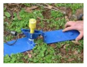
9. Continue inserting the probe into the ground with gentle blows of the *sledgehammer*, whilst holding the top of the probe steady with one hand, using the *EasyAG 80 dolly*, until the base of the *top cap* is level with the ground. This will place the top *sensor* at 10 cm (3.9 inches) below the ground surface. Remove the *EasyAG 80 dolly*.
