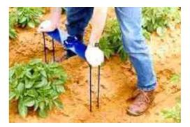
10. Using a *sledgehammer* alternately beat the *stabilization plate* at the points provided to force it doser to the ground. Do not beat continuously on any one side in advance of the other. The aim is to achieve a situation where the pins are near parallel in the ground.
