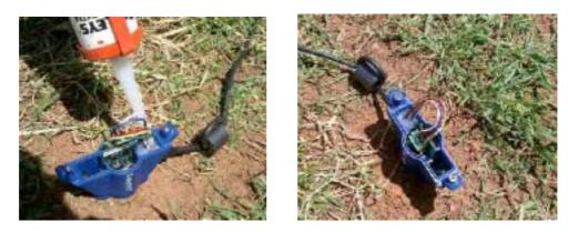
3. Ensure that the sealing gasket on the top cap is **clean**, in **good condition** and positioned correctly, and replace the *lid* of the *top cap*. Tighten the screws evenly completely to ensure an effective seal.
