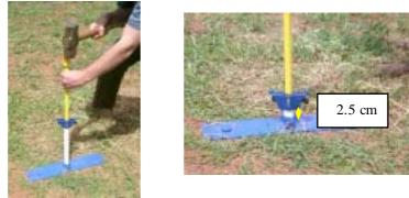
**Note**: This clearance height is important. If you hammer the probe in too far you will not be able to lift the stabilization plate off the long stabilization plate pins.
