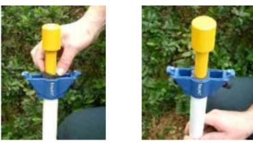
5. Continue inserting the *probe* by hammering on the insertion dolly with a *sledgehammer* until there is a 2.5 cm (1 inch) gap between the base of the *top cap* and the edge of the *stabilization plate* tube guide.
