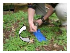
4. Carefully lift the AMS soil sampler directly out of the ground. To remove the soil collected in the soil sampler, simply beat on its side with the hand or foot. The design is such that the soil core taken is slightly compressed, and of a lesser internal diameter than the soil sampler itself. In heavier textures, the soil sampler deaning tool is used to clear the soil sampler by simply screwing it into the compressed soil. The extracted soil should be deposited away from the probe site.
