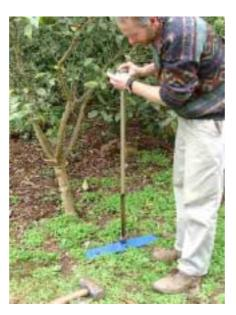
2. Using a *sledgehammer*, beat the *AMS soil sampler* into the ground until the beating head is just above the *stabilization plate*. (While it is preferable to go all the way in one insertion, successful installation may be possible in heavier soils with 2 insertions). Ensure accurate blows are made such that lateral deflection of the soil sampler is minimized. Do not compress the soil with the final blow.
