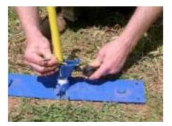
6. Remove the stabilization plate wing nuts.
