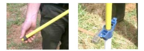
4. Continue inserting the *probe* by hammering on the insertion dolly with a *sledgehammer* until there is a 2.5 cm (1 inch) gap between the base of the *top cap* and the edge of the *stabilization plate* tube guide.
