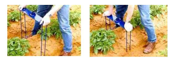
4. Using a *sledgehammer* alternately beat the *stabilization plate* at the points provided to force it doser to the ground. Do not beat continuously on any one side in advance of the other. The aim is to achieve a situation where the pins are near parallel in the ground.
