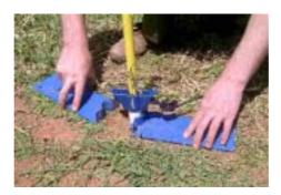
8. Continue inserting the probe into the ground with **gentle** blows of the *sledgehammer* using the *EasyAG 50 dolly*, until the base of the *top cap* is level with the ground. This will place the top *sensor* at 10 cm (3.9 inches) below the ground surface. Remove the EasyAG 50 dolly.
