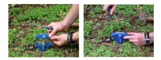
4. Tighten the *FairRite bead* and into position and tighten the cable gland. The probe is now installed and upon connection to the data logger is ready for use.
