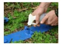
2. Insert the assembled complete *probe* into the *stabilization plate* and push it into the ground in a single gentle movement as far as it will go. Do not cause undue inflection of the access tube, as this will destroy the integrity of the installation.
