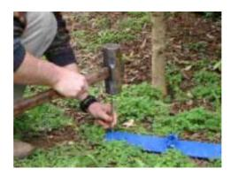
4. Put the soil sampler *polyguide* in place. The *stabilization plate* is now ready for insertion of the *AMS* soil sampler.
