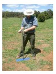
2. Using a *sledgehammer*, beat the *AMS soil sampler* into the ground until the bottom of the beating head sits 25 cm above the *stabilization plate*. **Note**: While it is preferable to go all the way in one insertion, successful installation may be possible in heavier soils with 2 insertions. Ensure accurate blows are made such that lateral deflection of the soil sampler is minimized.
