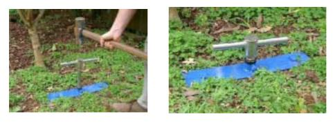
**Warning** Do not compress the soil such that normal water infiltration is inhibited
