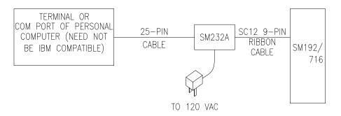
5.1-4 Storage Module Connected With SM232A
