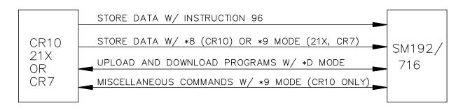
Figure 1.4-1 Operation with Current CR10, 21X, and CR7
