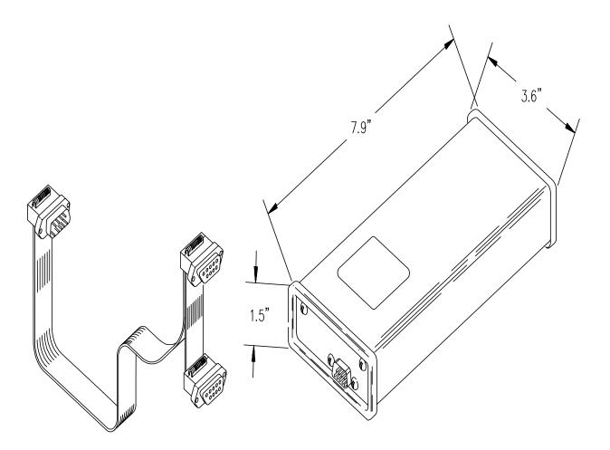
FIGURE 1.2-1. Storage Module and SC12 Cable
