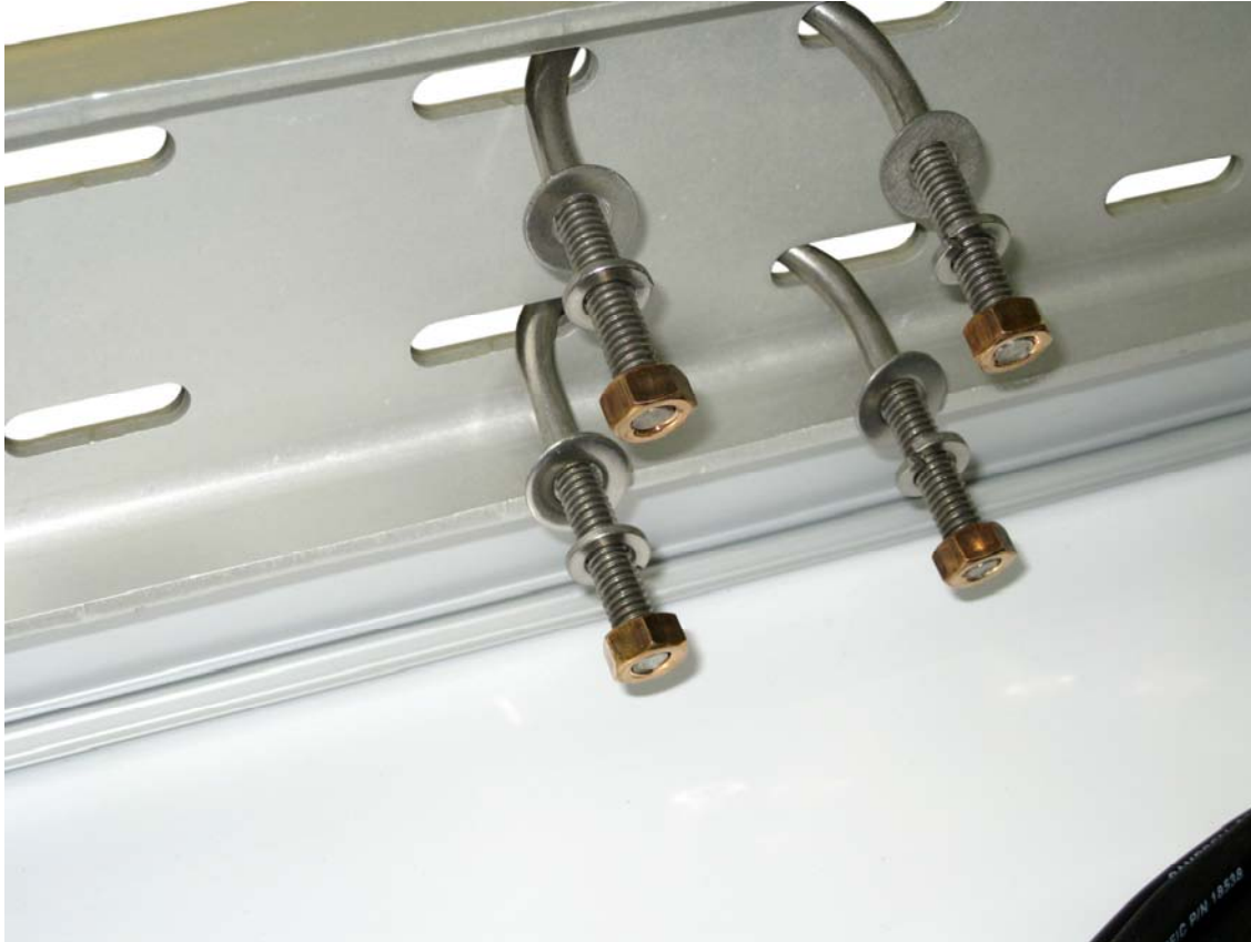
FIGURE 10. Lock Washers and Flat Washers are Used to Secure the Two 5/16-18 x 2.0 U-Bolts to the Solar Panel Mount
