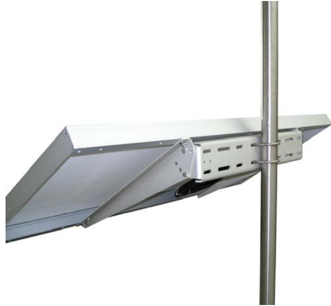
FIGURE 12. SP70 is Mounted to a Pole Using Two 5/16-18 x 2.0 U-Bolts
