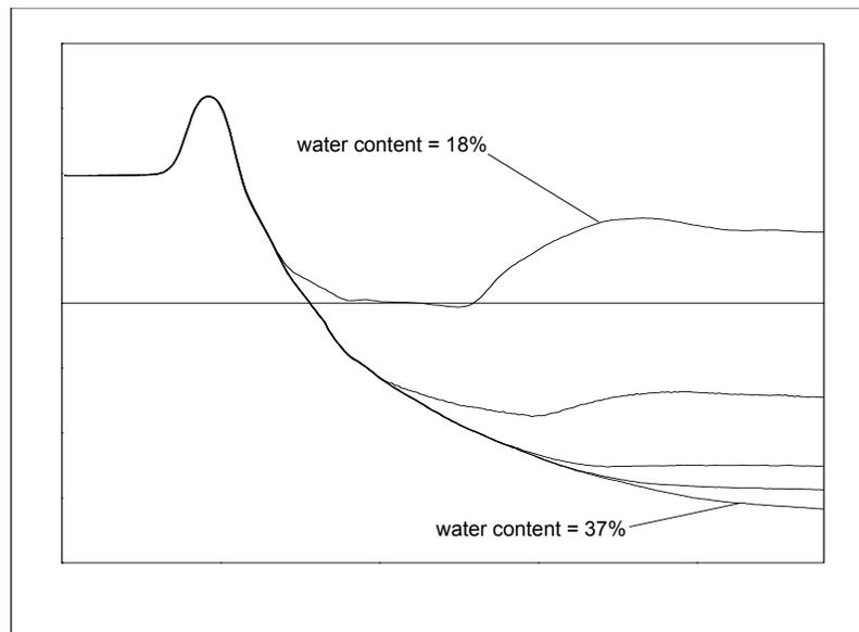
FIGURE 7-3. Waveforms collected in a sandy loam using CS610 probe with RG8 connecting cable. Volumetric water content values are 10, 18, 26, 30 and 37%. Solution electrical conductivity is  $10.2 \text{ dS m}^{-1}$ .
