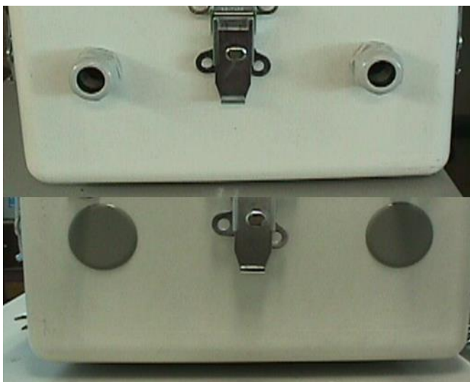
FIGURE H-5. Cryocooler feedthrough holes with grommets (above) and plugs (below)
