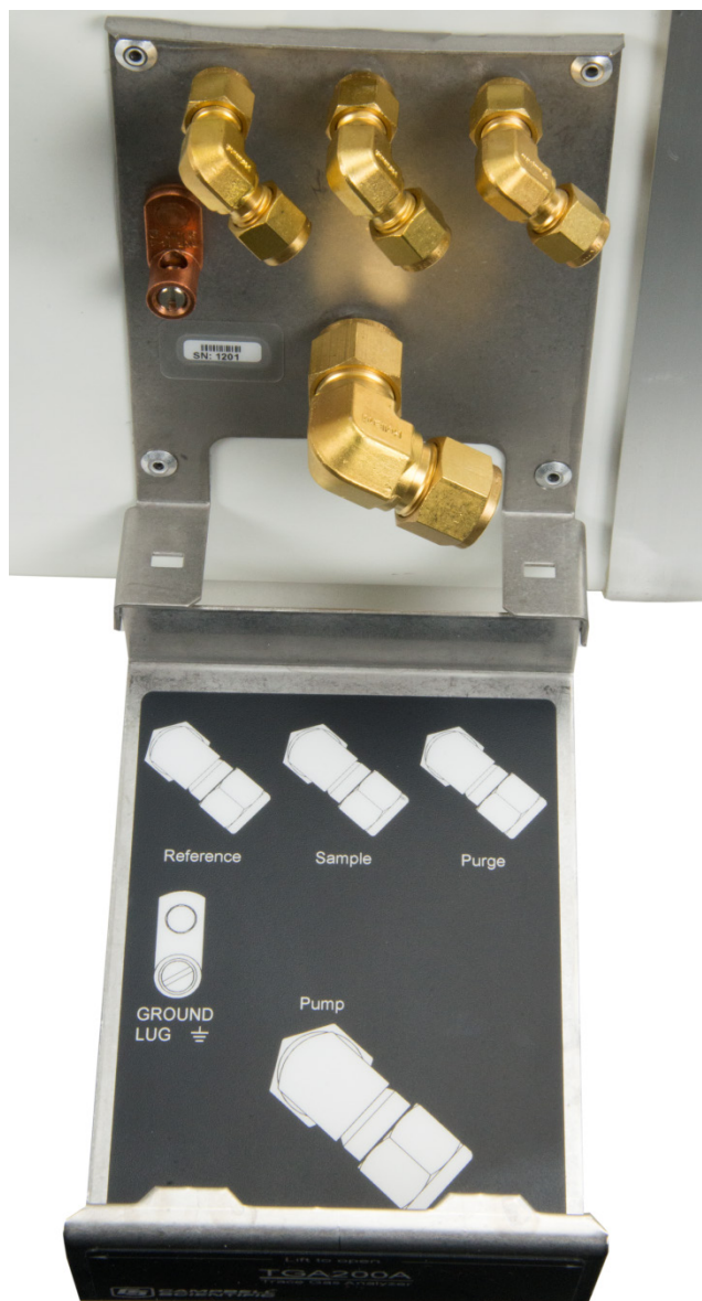
FIGURE 6-7. Plumbing connections located under feedthrough cover of TGA200A
