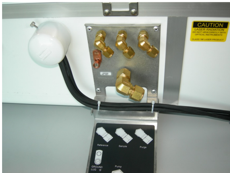
FIGURE 6-12. Routing of SDM and power cable through TGA200A feedthrough bracket
