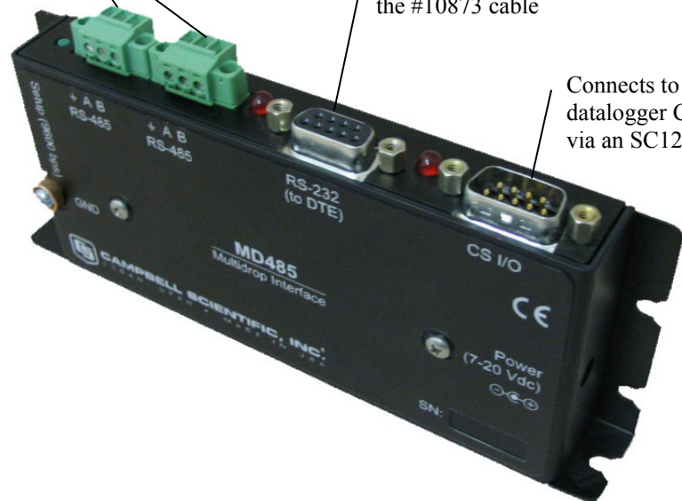
FIGURE 3.3-5. You can configure any two types of interface ports (RS-485, RS-232, and CS I/O) to be used at a time.
