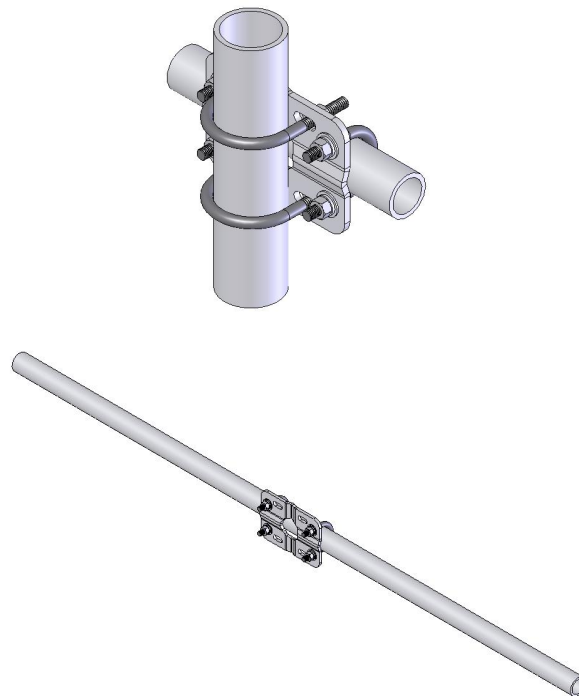
FIGURE 2-9. CM210 crossarm-to-pole bracket (top) is included with the crossarm for attaching the crossarm to the tripod's mast.
