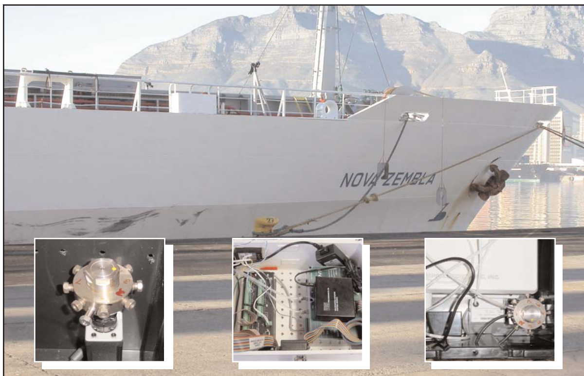
The instrumented citrus transport ship sits at the dock awaiting departure. Inset photos: the rotary valve, datalogger, CO 2 analyzer, and tubing.
