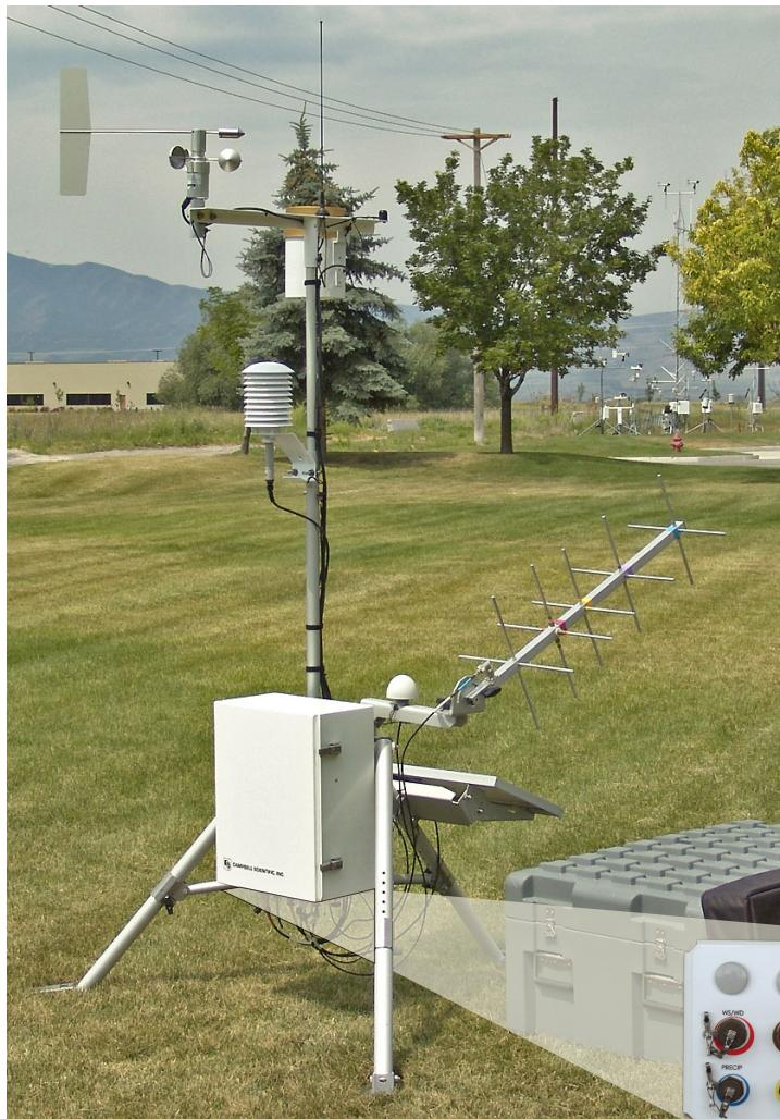
Campbell Scientific's RAWS-F (Remote Automated Weather Station for Fire Weather) is ideal for prescribed burns or other temporary installations. This lightweight, pre-configured station can be set up in as little as 10 minutes—without tools. An aluminum environmental enclosure houses a 12-V rechargeable battery and a CR1000M Module; in turn, the enclosure mounts to a 6-ft tripod. The battery is recharged with either a solar panel or AC power.
