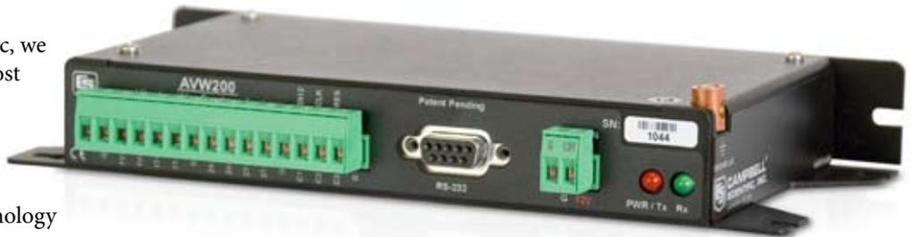
enough, it can render data useless. The new AVW200 interface module applies a new method for measuring the sensor's frequency. The traditional method uses a time-domain approach. The natural or resonant frequency at which the wire is oscillating is determined by exciting the wire with an AC excitation, stopping the excitation, and then measuring time between response pulses.
