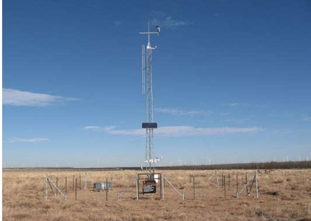
sure numerous factors of wind, air temperature and humidity, sunlight, soil temperature and water content at multiple depths, precipitation, and barometric pressure.
