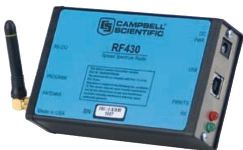
To make it easier to connect to newer computers, we are releasing three new spread-spectrum radios with USB ports. The new RF430 (900-MHz), RF431 (922-MHz), and RF432 (2.4-GHz) radios are functionally the same as our RF401 series. The difference between the two is that the RF430 series has both USB and RS-232 ports, while the RF401 series has RS-232 and CS I/O ports.
