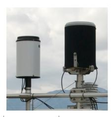
ampbell Scientific now offers the 52202 and CS700H heated rain gages. The 52202 is manufactured by R.M. Young and is intended for standard applications. It measures precipitation in 0.004-in. increments, with an accuracy of 3 percent for up to 2 in./hr.
