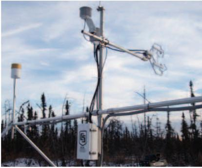
inner parts of the analyzer in extreme cold while maximizing power-use efficiency. The EC150 also provides field-based CO<sub>2</sub> zero/span capability using only the datalogger, which allows uninterrupted monitoring, even in this very remote Alaska location.
