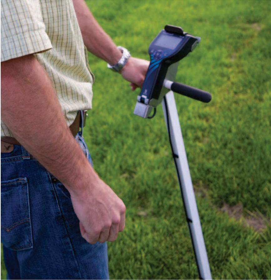
The HS2P HydroSense II Pole, Campbell Scientific's newest HydroSense soil-water measurement product, facilitates both the insertion of the probe into the soil and its removal. The HS2P has an aluminum insertion pole that is lightweight, yet sturdy enough to handle repeated soil insertions and removals. Because the pole is used
