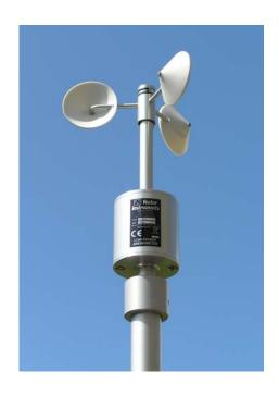
The A100LK and A100L2 low power anemometers are precision instruments which easily interface with Campbell Scientific dataloggers to give accurate measurements of wind run or mean wind speed. Rotation of the 3-cup rotor is electronically converted to pulse output signals proportional to wind speed.
