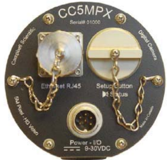
The connectors have metal caps that are chained to the camera.
