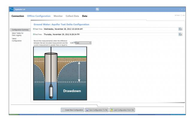
HydroSci software simplifies the process of configuring the CRS451. Users can configure the CRS451 to monitor surface water, ground water, or a standard pump test (shown above).
