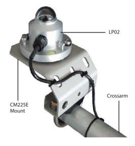
To attach the CM225E to a CM202, CM204, or CM206 crossarm, place the U-bolt in the holes on the bottom of the bracket (shown). If the CM225E is attached to a mast, place the U-bolt in the holes in the side of the bracket.
