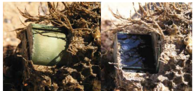
Biological fouling on an OBS500 probe after 86 days of deployment in the Atlantic Ocean near Savannah, Georgia. A closed sensor (far left) and opened sensor are shown.
