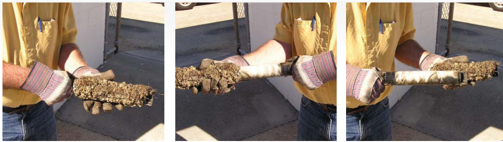
The OBS500 has a plastic sleeve option that can simplify clean up. The three above photographs show the sleeve being removed.
